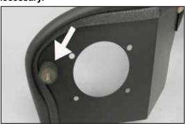
12. Install one of the supplied rubber mounted stud onto the heat shield as shown and secure with the provided hardware.
