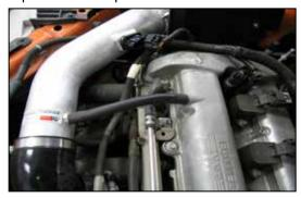
24. Install the crankcase vent hose onto the vent fitting on the valve cover.
