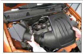
8. Lift the intake tract assembly off of the throttle body and then remove the complete assembly from the vehicle.
