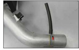
20. Install the provided crankcase vent hose onto the K&N® intake tube as shown.
