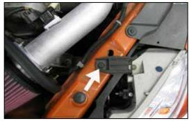
22. Remove the headlight mounting bracket bolt shown.
