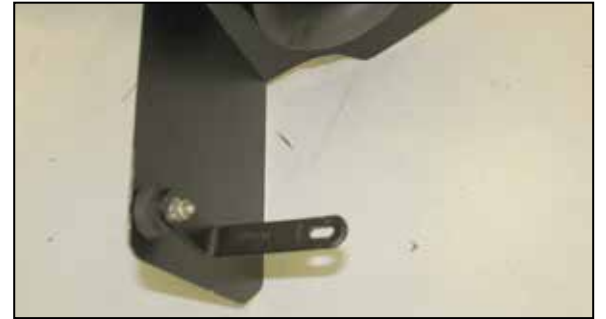
21. Install the rubber mounted stud and small "L" bracket onto the heat shield using supplied hardware. Do not tighten completely at this time.
