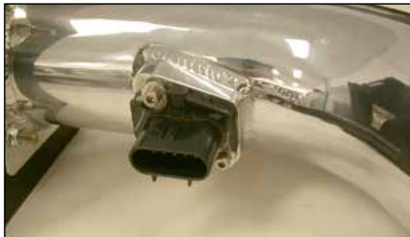
17. Install the mass air sensor onto the K&N® intake tube with provided hardware.
