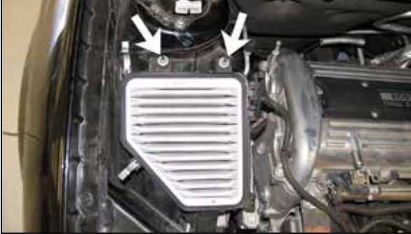
10. Loosen and remove the two airbox retaining nuts then remove the airbox from vehicle. NOTE: K&N Engineering, Inc., recommends that customers do not discard factory air intake.
