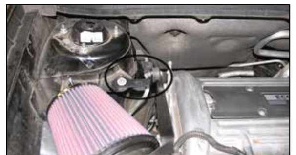
26. Align the heat shield bracket onto the stock airbox mounting stud and secure it with the stock bolt from step #10.
