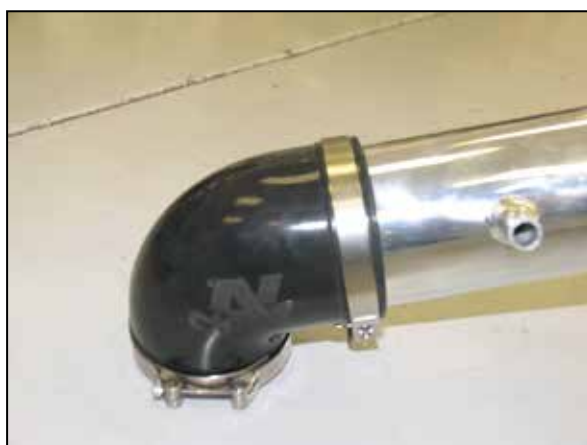
20. Install the silicone hose and hose clamps onto the intake tube as shown.
