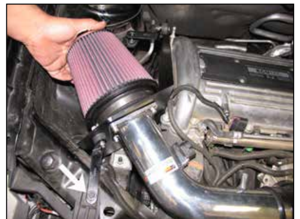
25. Align the heat shield bracket onto the head light mounting hole and secure it with stock bolt from step #12.
