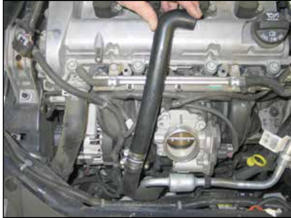
16. On models with air injection, attach the air injection hose assembly to the factory rubber air injection hose and secure with provided hose clamp.
