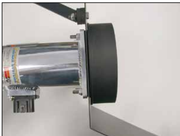
19. With the provided hardware, assemble the filter adaptor and gaskets onto the heat shield and intake tube as shown.
