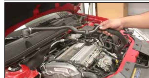
14. On models with air injection, disconnect the air injection pump plastic hard line from the air injection rubber hose.
