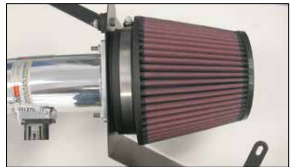
23. Secure the K&N® air filter onto the filter adaptor and secure with provided hose clamp. NOTE: Drycharger® filter wrap; part # RU-5147DK is available to purchase separately.
