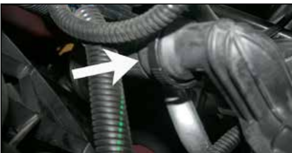
13. On models NOT equipped with air injection, install the provided cap onto the 1" vent fitting and secure with the provided hose clamp. NOTE: You may now proceed to step #17.
