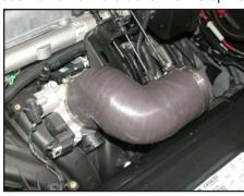
20. Install the silicone hose and hose clamps onto the throttle body as shown.
