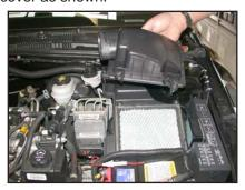
11. Loosen and remove the four air cleaner bolts to remove the air cleaner cover as shown.
