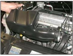
8. Pull upwards to remove the intake plenum as shown.
