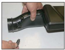
9. Remove the air temperature sensor from the intake tube as shown.
