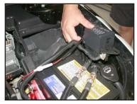
14. Disengage the plastic rivet and pull the fuse box upwards as shown.
