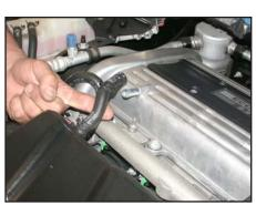
7. Remove the crankcase vent hose from the intake plenum as shown.
