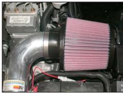
29. Install the K&N® air filter onto the K&N® intake tube and secure with the provided hose clamp as shown.
