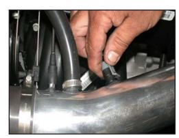
28. Reconnect the air temperature sensor electrical connection as shown.
