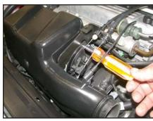
6. Loosen the hose clamp on the intake plenum at the throttle body as shown.
