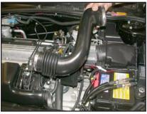
5. Loosen hose clamps and remove the stock intake tube as shown.
