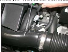
2. Disconnect the air temperature sensor electrical connection as shown.
