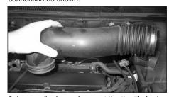
Loosen the hose clamps at the throttle body and at the mass air sensor, then, remove the stock intake tube as shown.
