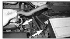
5. Remove the vent hose from the side of the lower air cleaner and valve cover.
