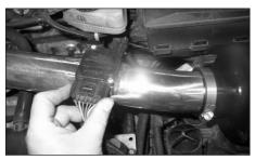
14. Reconnect the mass air sensor electrical connection as shown.
