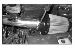
13. Install the K&N Filtercharger onto the K&N Typhoon intake tube and tighten with the provided hose clamp as shown.
