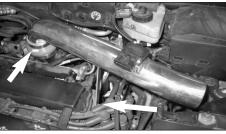
11. Install the K&N Typhoon intake tube into the silicone hose then line up the bracket with the ignition bracket and secure with the bolt from step 10 and tighten the hose clamps.
