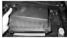
4. Remove the four bolts that secure the air cleaner cover, then remove the cover and filter as shown.
