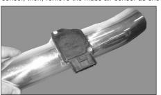
9. Install the mass air sensor into the K&N Typhoon intake tube using the stock bolts from step 8.
