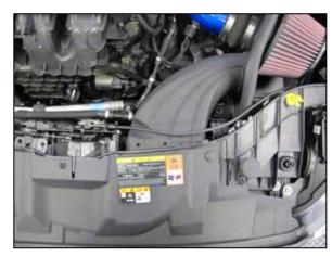
20. Install the K&N® fresh air duct onto the core support and into the K&N® heat shield.
