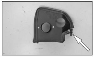
12. Install the mounting post from the previous step onto the K&N® heat shield as shown.
