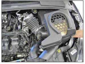
6. Lift and dislodge the air box from its mounting grommets and then remove the air box from the vehicle.
