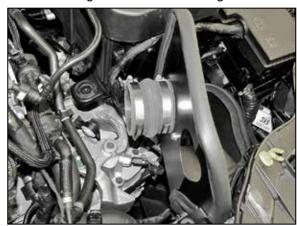
14. Install the provided coupler hose (087212) onto the filter adapter and secure with the provided hose clamp.
