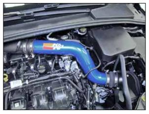
17. <u>Install the K&N intake tube</u> into the factory coupler and then into the K&N® coupler, adjust the tube for best fit and then secure with the provided hose clamps.
