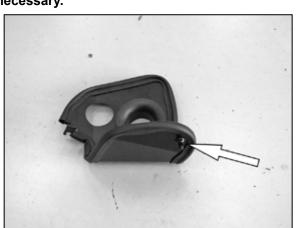
10. Install the heat shield mounting stud onto the heat shield and secure with the provided hardware.
