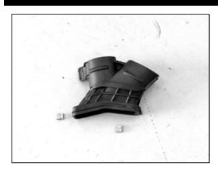
22. Remove the two clips from the factory inlet air hose.
