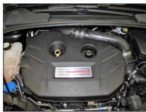
2. Lift off the engine cover and remove it from the vehicle.
