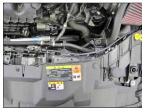
21. Using the K&N® Fresh air duct as a guide, mark the two hole locations onto the fresh air duct in the core support. Next remove the K&N® fresh air duct and drill two ¼"id holes into the factory fresh air duct in the core support at the marked locations.
