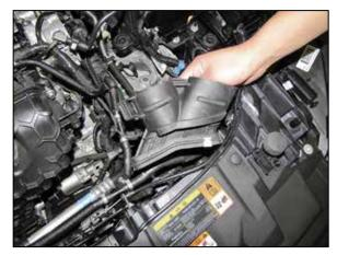
7. Remove the inlet air duct from the core support.
