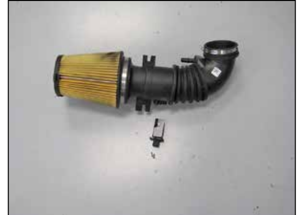
18. Remove the mass air sensor from the factory intake tube.
