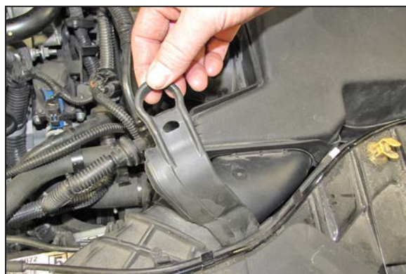
4. Release the rubber strap that secures the fresh air intake hose.
