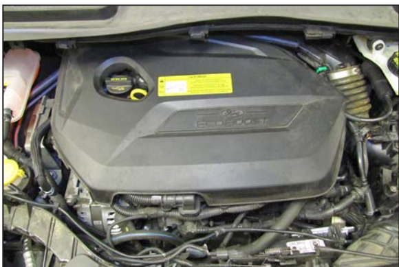
2. Lift up and remove the decorative engine cover.
