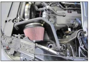
15. Install the K&N<sup>®</sup> air filter onto the adapter and secure with the provided hose clamp, then secure the heat shield and brackets to the air filter housing mounting location using the provided hardware. **NOTE: Drycharger<sup>®</sup> air filter wrap; part #**
