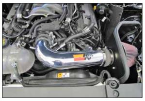
20. Install the K&N<sup>®</sup> intake tube into the hose at the filter adapter and then into the hose at the throttle body, adjust the tube and hoses for best fit and then secure with the provided hose clamps.
