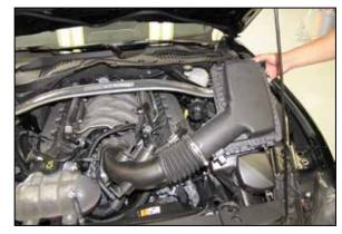
9. Loosen the hose clamp securing the intake tube to the throttle body and then remove the air filter assembly and intake tube from the engine compartment.
