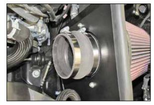
16. Install the provided hump coupler (08699) onto the filter adapter and secure with the provided hose clamp. 21. Connect the crank case vent, EVAP vent and idle by pass lines to the quick disconnect fittings installed into the K&N<sup>®</sup> intake tube. NOTE: On vehicles not equipped with an EVAP vent line, install the provided caplug #08215 onto the quick disconnect fitting.
