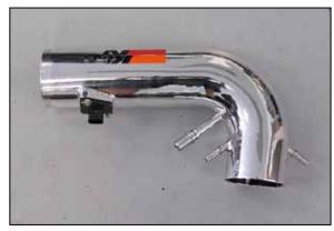
19. Install the mass air sensor into the K&N $^{\odot}$  intake tube and secure with the provided hardware.
