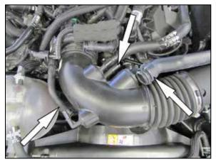
4. Depress the locking tabs and then disconnect the crank case vent hose and the EVAP vent hose. Then release the spring clamp and disconnect the sound tube from the intake tube. **NOTE: Some vehicles are not equipped with the EVAP vent hose.**  5. Cut the clamp that secures the sound tube/ chamber to the sound drum and then disconnect the sound tube/chamber from the sound drum.
