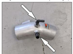
10. Install the two provided vent fittings into the K&N® intake tube as shown.
