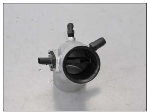
15. Install the venturi into the K&N® intake tube as shown.
