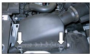
5. Release the two clips securing the upper air box to the lower air box.
