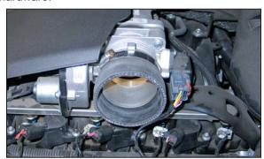
17. Install the provided silicone hose onto the throttle body as shown and secure with the provided hose clamp.
