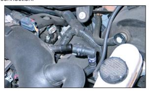
3. Disconnect the crank case vent hose from the intake tube.
