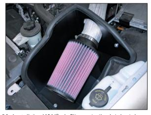
20. Install the K&N® air filter onto the intake tube and secure with the provided hose clamp. RC-5106DK is available to purchase separately.
