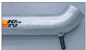
15. Install the provided crank case vent fitting into the  $K\&N^{\tiny \circledcirc}$  intake tube as shown.
