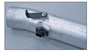
16. Install the tube mounting bracket (07805) onto the K&N® intake tube as shown using the provided hardware.
