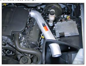
18. Install the intake tube into the heat shield and then into the silicone hose at the throttle body, secure the tube bracket to the heat shield with the provided hardware. Secure the intake tube to the silicone hose with the provided hose clamp.
