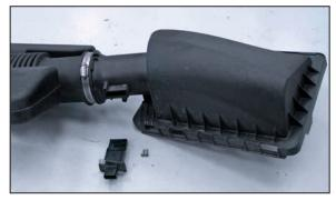
13. Remove the two screws securing the mass air sensor to the factory air box and then remove the sensor from the air box.
