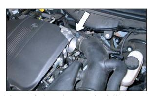
4. Loosen the hose clamp securing the factory intake tube to the throttle body and then disconnect the intake hose from the throttle body.
