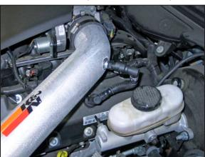
19. Connect the crank case vent hose to the fitting installed into the K&N® intake tube as shown.
