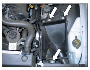
7. Remove the three nuts securing the lower air box into the engine compartment.
