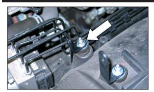
10. Install the provided heat shield mounting bracket (070066) onto the lower most rear factory air box mounting stud as shown.
