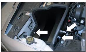
12. Install he heat shield assembly into the engine compartment and secure to the previously installed brackets and the forward factory air box mount with the provided hardware.
