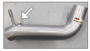
16. Install the provided NPT fitting into the K&N® intake tube as shown.
