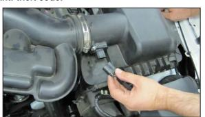
2. Disconnect the mass air sensor electrical connection.
