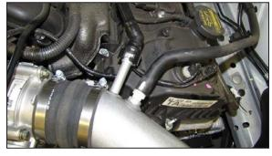
20. Connect the crank case vent hose and EVAP hose to the K&N® intake tube as shown.
