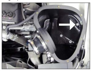
15. Install the K&N® air box onto the inner fender so the mounting grommets are inserted into the mounting holes and then secure the air box with the provided hardware.
