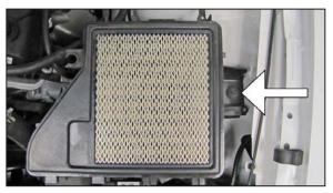
7. Remove the bolt that secures the lower air box to the inner fender shown.
