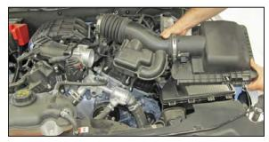
6. Remove the upper air box/tube assembly from the vehicle.
