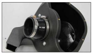
12. Install the provided silicone hose (08724) onto the K&N® filter adapter and secure with the provided hose clamp.
