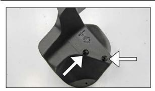
10. Install the two provided mounting studs to the bottom of the K&N<sup>®</sup> air box as shown and secure with the provided hardware.
