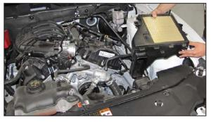
8. Remove the lower air box housing from the vehicle.
