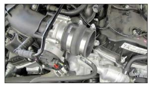
9. Install the provided silicone hose (08696) onto the throttle body and secure with the provided hose clamp as shown.
