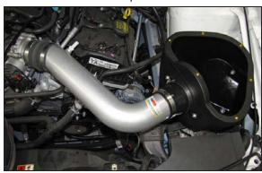
19. Install the K&N® intake tube into the silicone hose at the throttle body and then into the silicone hose on the filter adapter, secure the intake tube with the provided hose clamps.
