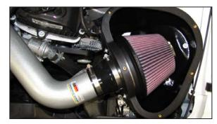
21. Install the K&N® air filter onto the filter adapter and secure with the provided hose clamp.
