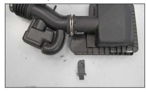
17. Remove the two screws securing the mass air sensor into the factory air box and then remove the mass air sensor.
