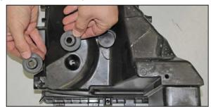
13. Remove the factory air box mounting grommet from the factory lower air box housing.
