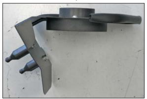
11. Install the filter adapter onto the heat shield and secure with the provided hardware.
