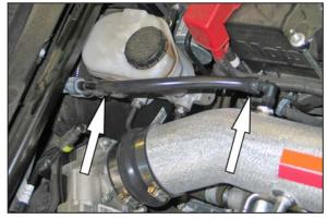
21. Connect the provided EVAP hose onto the 90° vent fitting installed in the K&N® intake tube, then connect the open end to the EVAP check valve as shown.
