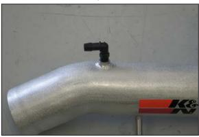
16. Install the provided 90° NPT vent fitting into the  $K\&N^{@}$  intake tube as shown.
