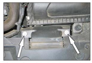
7. Remove the two bolts shown that secure the fresh air duct to the core support.
