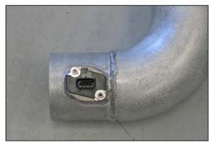
15. Install the mass air sensor into the K&N® intake tube and secure with the provided hardware.
