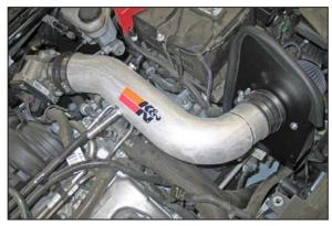
19. Install the K&N® intake tube assembly into the hose at the throttle body and then onto the filter adapter and secure with the provided hose clamp.
