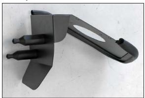
10. Install the heat shield mounts onto the heat shield and secure with the provided hardware.
