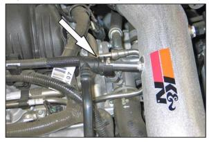
20. Connect the crankcase vent hose to the quick connect fitting on the K&N® intake tube.
