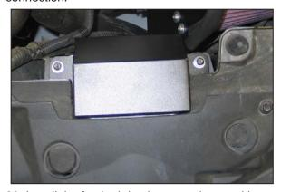
23. Install the fresh air intake scoop into position and secure to the heat shield and core support with the provided hardware.
