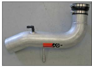
18. Install the provided silicone hose (084091) onto the K&N® intake tube as shown and secure with the provided hose clamp.
