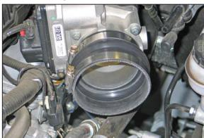
17. Install the provided silicone hose (084079) onto the throttle body and secure with the provided hose clamp.
