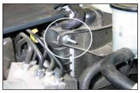
13. Remove the Left upper fan shroud mounting bolt shown.
