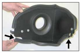
12. Install the shorter 20" section of edge trim onto the heat shield as shown.
