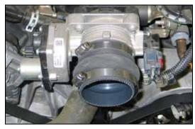
15. Install the provided hump hose (08421) onto the throttle body and secure with the provided hose clamp.
