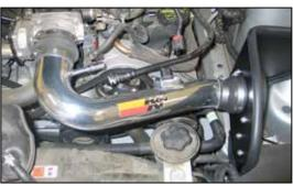
19. Install the K&N® intake tube into the silicone hose on the filter adapter and then into the silicone hose at the throttle body. Secure the intake tube with the provided hose clamps.
