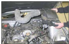
6. Remove the air box assembly from the vehicle. NOTE: K&N Engineering, Inc., recommends that customers do not discard factory air intake.
