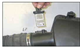
17. Remove the two screws which secure the mass air sensor and then remove the mass air sensor from the stock air box.
