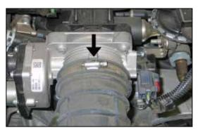
4. Loosen the hose clamp which secures the stock intake tube to the throttle body.
