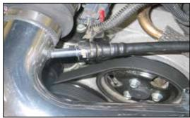
20. Connect the crank case vent hose to the K&N<sup>®</sup> intake tube as shown.
