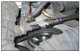
3. Release the locking ring and then disconnect the crank case vent tube.
