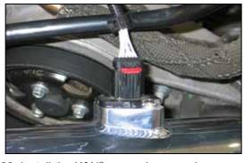
22. Install the K&N® mass air sensor harness extension into the factory wiring harness and then connect the open end into the mass air sensor.
