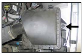
5. Remove the bolt which secures air box to the inner fender.
