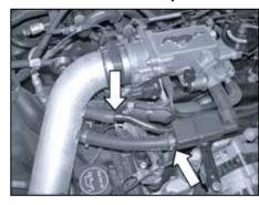
26. Reconnect the vent hoses to the K&N<sup>®</sup> intake tube as shown and tighten hose clamps.
