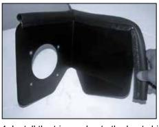
14. Install the trim seal onto the heat shield. NOTE: Some cutting and trimming will be necessary to achieve best fit.
