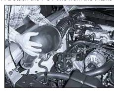
8. Remove the entire air intake assembly.
