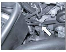
25. Slide the brackets onto the stud from step 13 and secure with the factory nut.
