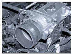
17. Install the provided silicone hose and hose clamps onto the throttle body as shown.
