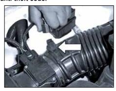
2. Disconnect the air temp sensor electrical connection.
