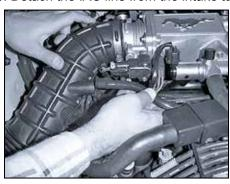
7. Detach the PCV line from the intake tube.
