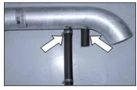
19. Install the provided hoses from the previous step onto the K&N $^{\otimes}$  intake tube and secure with the provided hose clamps as shown.
