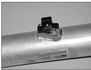
15. Install the mass air sensor into the K&N® intake tube with the factory mounting screws.
