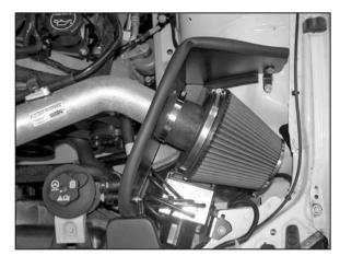
22. Install the K&N® air filter assembly onto the K&N® intake tube as shown and secure with the provided hose clamp.
