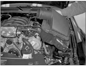
6. Remove the airbox assembly as shown.
