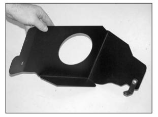
9. Install the "L" bracket (070812) onto the rear of the heat shield as shown with the provided hardware.
