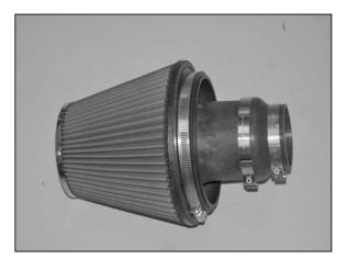
21. Install the silicone hose onto the air filter assembly and secure with the provided hose clamp as shown.
