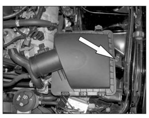
5. Remove the airbox mounting bolt shown.
