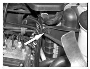
12. Remove the radiator fan shroud mounting bolt shown.
