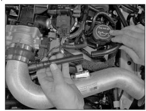
18. Using a razor blade cut the crankcase vent tube 6" from the end as shown.
