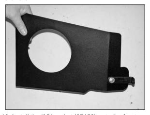
10. Install the "L" bracket (07158) onto the front of the heat shield as shown with the provided hardware.
