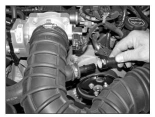
3. Rotate the green locking tab clockwise and then disconnect the crankcase breather hose from the intake tube.
