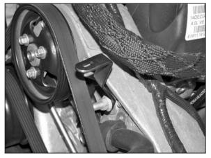
8. Install the tube-mounting bracket onto the power steering mounting bracket stud and secure with the nut removed in step #7.
