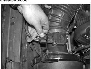
2. Disconnect the mass air sensor electrical
