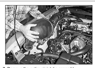
7. Remove the entire air intake assembly. NOTE: K&N Engineering, Inc., recommends that customers do not discard the factory air intake.
