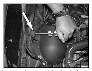
4. Loosen and remove the bolt that retains the air
