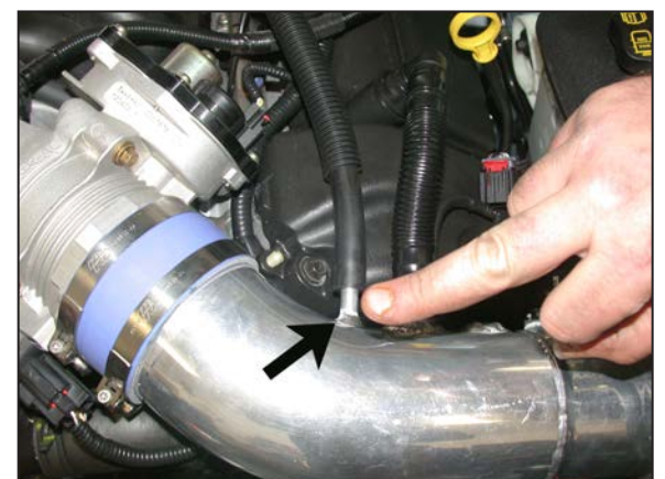
20. Install the small vent hose onto the intake tube as shown.
