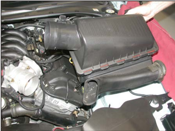
9. Pull up firmly on the air box to dislodge it from the retaining pin, and then remove the air box from the vehicle.
