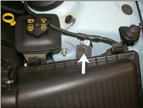
8. Remove the air box retaining bolt shown.
