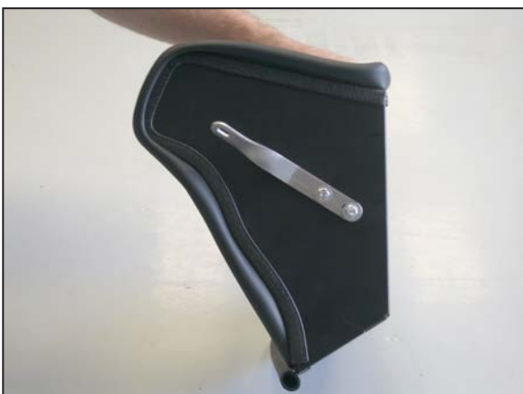
11. Install the heat shield mounting bracket (010083) onto the heat shield as shown with the provided hardware.
