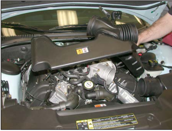
7. Remove the stock intake tube assembly from the vehicle.
