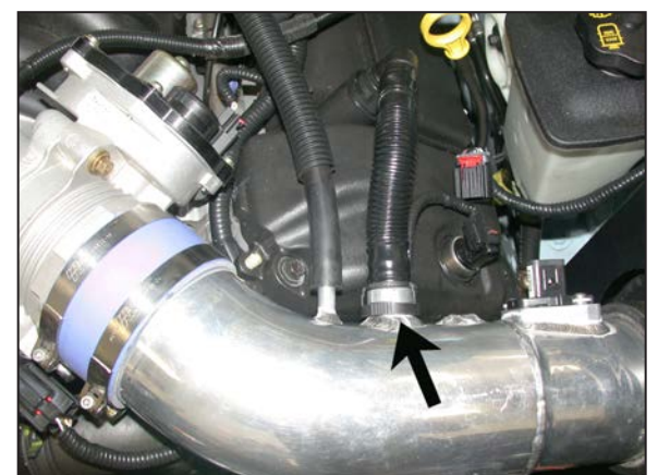
21. Install the large vent hose onto the intake tube as shown.
