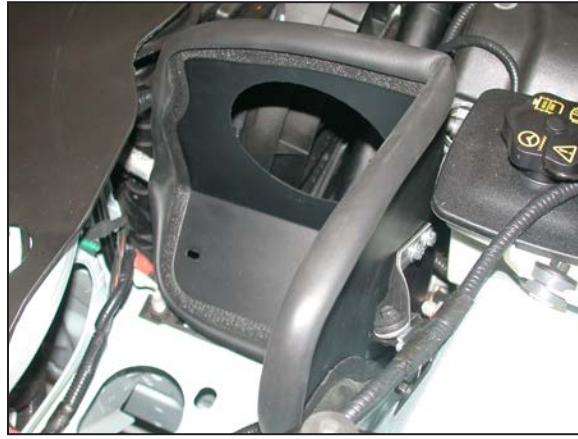
12. Install the heat shield into the vehicle and secure the bracket to the factory air box mount with the factory bolt removed in step #8.
