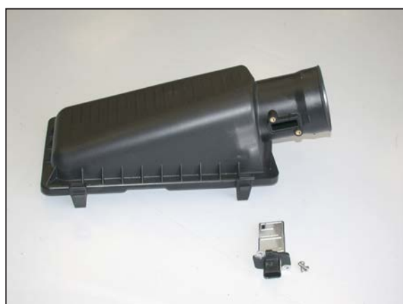
16. Using the "TORX" wrench provided, remove the mass air sensor from the air box lid as shown.
