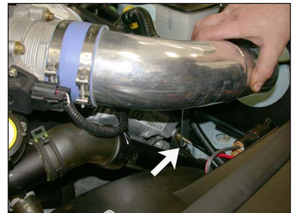
18. Install the intake tube assembly into the silicone hose at the throttle body and slide the bracket onto the stock bolt as shown.
