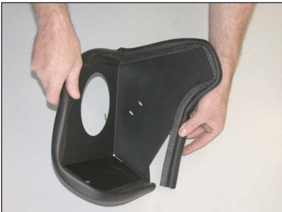
10. Install the provided edge trim onto the heat shield as shown.
