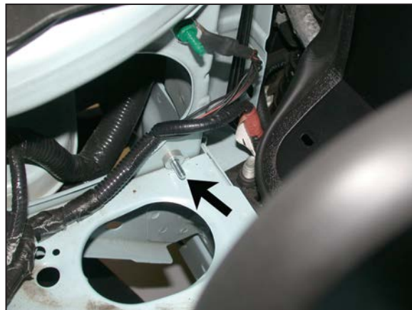
13. Install the provided 6mm bolt through the factory hole in the core support and then install the provided spacer onto the bolt as shown.
