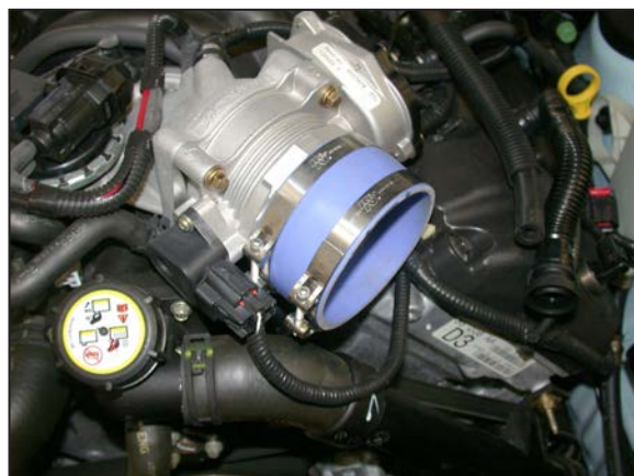
15. Install the provided silicone hose (08698) onto the throttle body and secure with the provided hose clamp.
