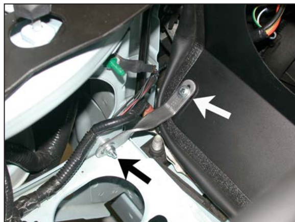
14. Install the provided heat shield bracket (010084) onto the bolt installed in step #13, and then fasten the bracket to the heat shield with the provided hardware.
