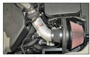
18. Install the K&N® intake tube into the hose at the plenum and then into the hose at the filter adapter and then secure with the provided hose clamps.
