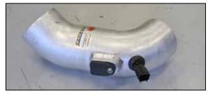
17b. Install the provided grommet into the hole drilled. Then remove the O-ring from the sensor and install the sensor into the grommet.
