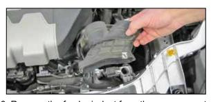
$\ensuremath{\text{6}}.$  Remove the fresh air duct from the core support as shown.
