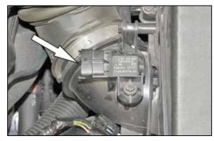
2. Disconnect the pressure sensor electrical connection.
