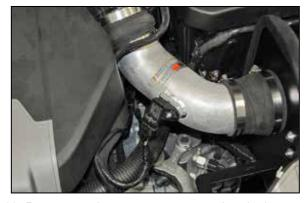
19. Reconnect the pressure sensor electrical connection.
