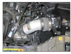
26. Install the K&N® intake tube completely into the silicone hump hose and then set the complete assembly onto the heat shield base.
