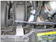
32. Disconnect the hood release cable from the hood latch.
