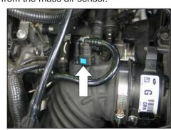
3. Depress the blue locking tab and then disconnect the EVAP vent line.
