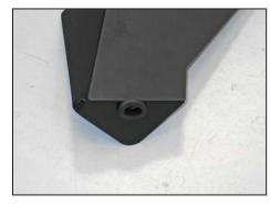
33. Install the provided 7/8"OD grommet into the K&N® fresh air plate as shown.
