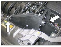
35. Install the 30" long section of edge trim onto the fresh air plate and heat shield as shown. Some trimming of the edge trim will be necessary.
