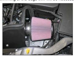
36. Install the  $K\&N^{\otimes}$  air filter and secure with the provided hose clamp.
