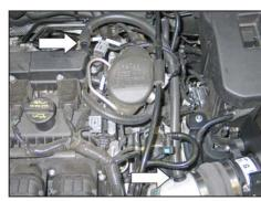
28. Install the provided silicone vent hose onto the 90° vent fitting in the K&N® intake tube and attach the open end to the valve cover port as shown.
