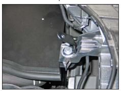
18. Using the provided hardware, secure the provided bracket (083161) to the fresh air intake scoop mount and the rubber mounted stud on the heat shield base.
