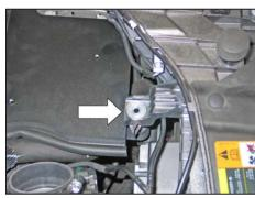
17. Place the provided fender washer onto the fresh air intake scoop mount as shown.
