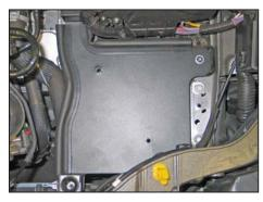
16. Set the heat shield base into position on the air box mounts.
