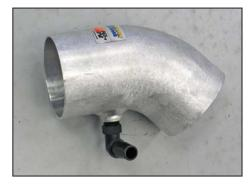
25. Install the 90° vent fitting into the K&N $^{\! \rm 8}$  intake tube as shown.
