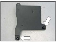
12. Install the two provided mounting studs onto the heat shield using the provided hardware.
