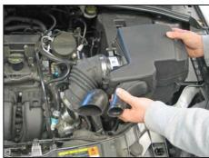
8. Lift up the air box assembly to release it from the mounting grommets; remove the air box from the vehicle.
