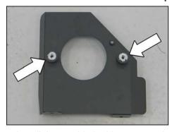
19. Install the provided rubber mounted studs onto the heat shield as shown.
