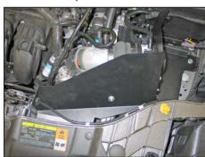
34. Pass the hood release cable through the grommet installed into the K&N® fresh air plate and then secure the fresh air plate to the heat shield and mounting bracket with the provided hardware. Reinstall the hood release cable to the hood latch.
