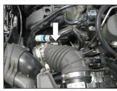
6. Loosen the hose clamp securing the intake tube to the throttle body.
