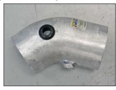
24. Install the provided 1.0"OD grommet into the K&N® intake tube as shown.
