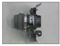
23. Install the provided hump hose (08421) onto the mass air sensor as shown and secure with the provided hose clamp.
