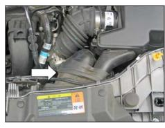
7. Release the rubber strap securing the fresh air intake scoop to the duct.
