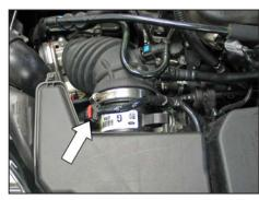
2. Release the red locking tab and then disconnect the mass air sensor electrical connection. Also unhook the mass air sensor wiring harness clip from the mass air sensor.
