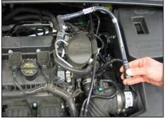
5. Disconnect the crank case vent hose from the valve cover and then remove the vent hose from the vehicle.
