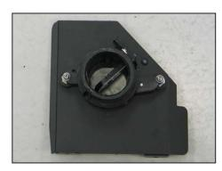
22. Secure the mass air sensor housing to the rubber mounted studs on the heat shield as shown using the provided hardware.
