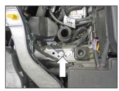
10. Remove the bolt shown securing the intake silencer to the inner fender; lift up to remove the intake silencer from the vehicle.
