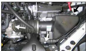
5. Release the three retaining clips securing the airbox lid and loosen the hose clamp at the throttle body.
