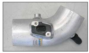
22. Install mass air sensor into K&N® intake tube and secure with the provided hardware as shown.
