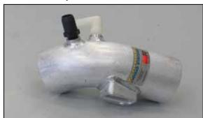
20. Install the 5/8" vent fitting into the K&N $^{\! 8}$  intake tube as shown.
