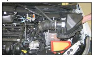
6. Remove factory intake hose and airbox lid from the vehicle.
