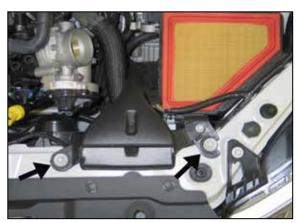
7. Remove the two bolts securing the lower airbox assembly to core support.
