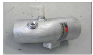
19. Install 90 degree vent fitting into the K&N® intake tube as shown.
