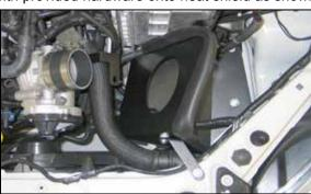
18. Install the heat shield into the vehicle as shown and secure with the provided hardware and the bolt removed in step #10.
