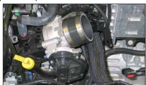
13. Install silicone hose (08440) with provided hose clamps onto the throttle body as shown.
