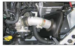
23. Install K&N® intake tube into silicone hose and aligning with tube mounting bracket and heat shield. Secure with provided hardware as shown.
