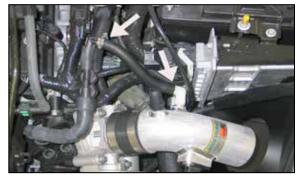
24. Install provided silicone hose onto the EVAP valve with provided hose clamp then onto 90° fitting on K&N® intake tube.
