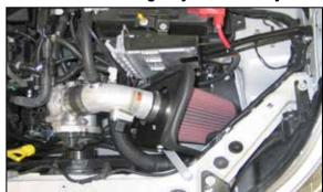
26. Install the K&N® filter onto K&N® intake tube secure with provided hose clamp as shown.
