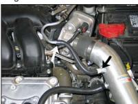
22. On vehicles equipped with an EVAP vent line, install the provided EVAP hose onto the port and then onto the ¼"NPT fitting installed into the K&N® intake tube as shown.
