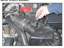
2. Disconnect mass air sensor electrical connection.
