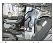
8. Remove the two bolts that secure the air box mount. Then remove the air box mount from the vehicle.
