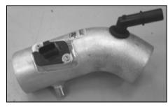
23. Install the provided grommet and stock crankcase vent fitting into the K&N® intake tube.
