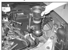
8. Loosen the hose clamp that fastens the mass air sensor housing to the air filter housing, then remove the mass air sensor housing.
