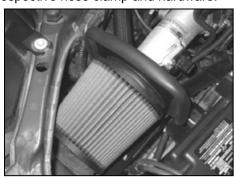
25. Install the K&N® air filter and fasten using the provided hose clamp.
