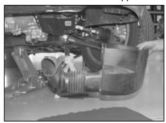
8d. On vehicles equipped with an airbox cover, lower the cover and remove it from the vehicle.
