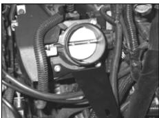
13. On 2008 and earlier models, Install the intake tube mounting bracket (06487) onto the throttle body as shown and secure with the factory mounting bolts from step # 12.
