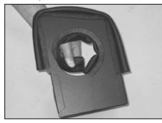
15. Install the edge trim onto the center portion of the heat shield.
