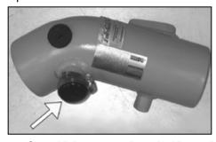
19c. On vehicles not equipped with an air injection pump, install the provided caplug onto the air injection fitting and secure with the provided hose clamp as shown.
