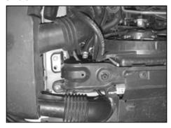
8c. On vehicle's equipped with an airbox cover, remove the two bolts which secure the cover to the frame rail, and the bolt which secures the intake snorkel to the radiator core support.
