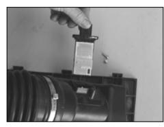
8a. Remove the two screws that fasten the mass air sensor to the factory airbox, then remove the mass air sensor.
