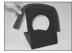
14. Install the edge trim onto the heat shield. **NOTE: Some trimming of the edge trim may be necessary.**
