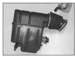
22. Remove the crankcase vent fitting from the stock intake tube.
