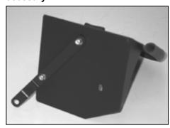
16. Install the heat sheild mounting bracket (06486) onto the bottom of the heat shield; fasten using the provided hardware.
