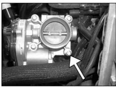
12a. On 2009 model vehicles, remove the lower rear throttle body mounting bolt shown.
