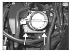
12. On 2008 and earlier models, remove the two lower throttle body bolts shown.
