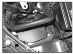
18. Place the heat shield into position onto the inner fender well heat shield mounting bracket and align the second heat shield bracket with the threaded hole in the inner fender. Fasten the heat shield using the provided hardware.
