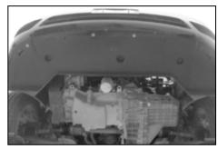
13c. On vehicle's that were equipped with the splash shield, reinstall with the bolts removed in step #8b.
