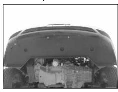
27. On vehicle's that were equipped with the splash shield, reinstall with the bolts removed in step #10a.
