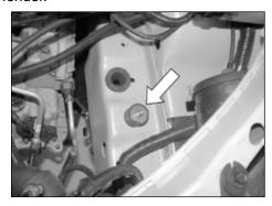
15. Install the supplied rubber mounted stud to the factory threaded hole as shown.
