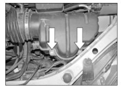
4. Loosen the two bolts, which secure the upper intake housing to the mass air sensor housing. NOTE: The two bolts do not separate from the upper intake housing.
