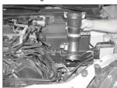
9. Pull firmly up and remove the mass air sensor assembly from the vehicle.
