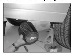
25. From underneath the vehicle, install the K&N® air filter onto the intake tube and tighten hose clamp completely.
