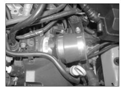
20. Install the supplied silicone hose and hose clamps onto the throttle body and tighten only the hose clamp over the throttle body.
