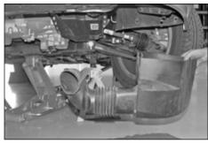
12. On vehicles equipped with an air box cover, lower the cover and remove it from the vehicle.
