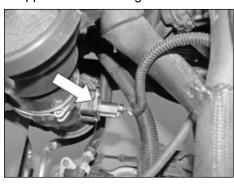
Depress the locking tab on the mass air sensor electrical connection and then disconnect the electrical connection.
