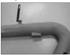
17. Install the supplied "L" bracket and hardware to the K&N® intake kit. Do not tighten completely. NOTE: Before installing the "L" bracket, inspect the inside of the tube for any debris, then clean the inside out with water and a towel. Inspect the tube one more time before proceeding to the next step.
