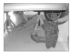
26. On vehicle's that were equipped with an air box cover, reinstall and secure with the bolts that were removed in step #11.
