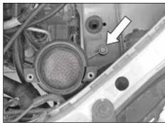
8. Remove the bolt, which secures the mass air sensor housing bracket to the inner fender.
