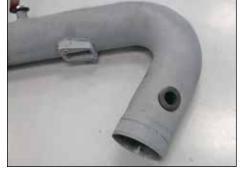
18. Install the supplied rubber grommet into the intake tube as shown.
