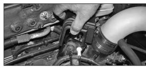
25. Reinstall the plastic throttle linkage cover as shown.
