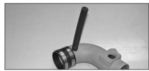
17. Install the provided silicone hose onto the vent on the K&N® Typhoon® intake tube as shown.
