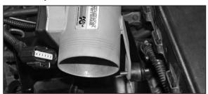
20. Line up the tube bracket with the rubber mounted stud and secure with the provided hardware as shown.
