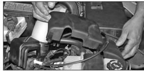
26. Reinstall the plastic coil cover as shown.
