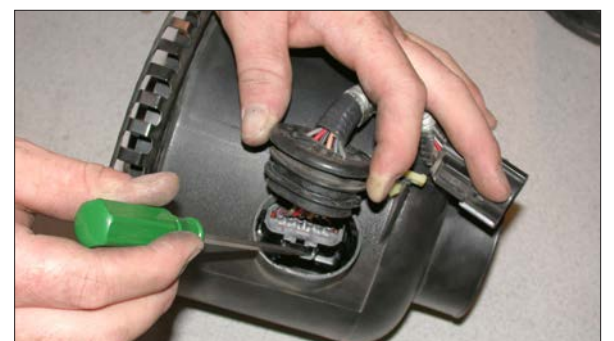
9. Pull the rubber boot back then depress the release tab to disconnect the mass air sensor electrical connection as shown.
