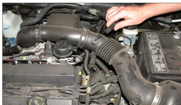
5. Remove the vent hose from the stock intake tube as shown.
