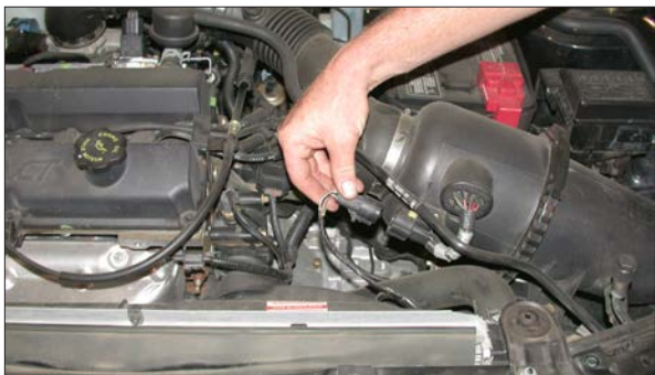
2. Disconnect the secondary mass air sensor electrical connection as shown.
