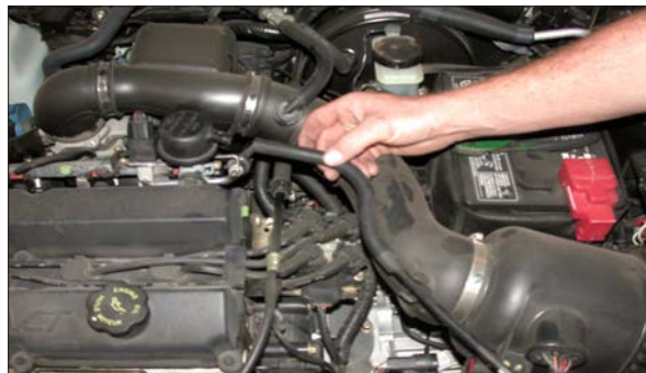
4. Remove the crank case vent hose from the breather on the cam cover as shown.
