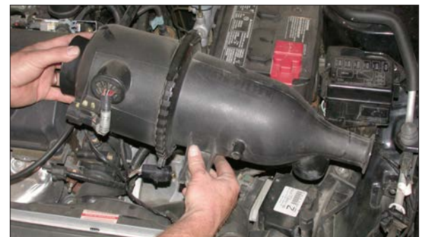
8. Pull firmly upwards to remove the air cleaner assembly as shown.
