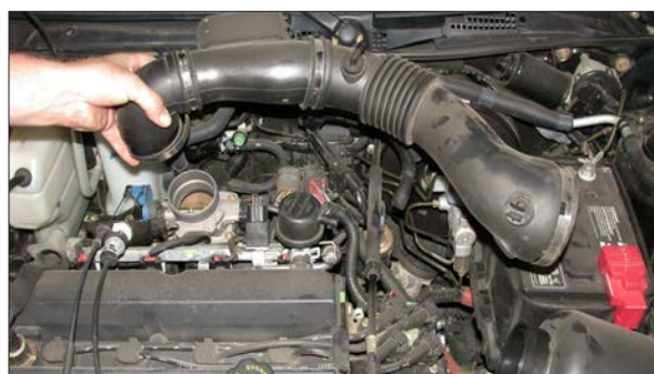
6. Loosen the hose clamp at the throttle body and at the mass air sensor, then, remove the stock intake tube as shown.
