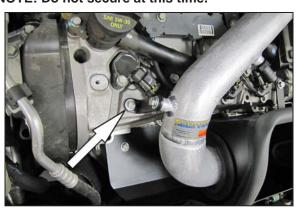
19. Install the provided tube mounting bracket (07158) onto the valve cover and intake tube with the provided hardware. Secure the hose clamps on the silicone elbow hose.
