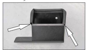
11. Install the 21" edge trim onto the heat shield as shown.
