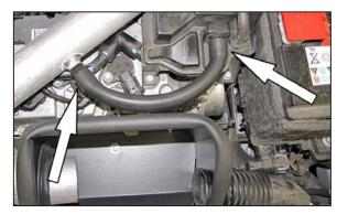
20. Attach the provided crank case vent hose to the fitting on the K&N® intake tube and the factory plenum.
