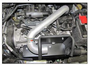
18. Install the K&N® intake tube into the heat shield and then into the silicone hose at the throttle body. **NOTE: Do not secure at this time.**
