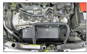
16. Set the heat shield onto the nut extensions, snap the fresh air duct into the heat shield and then secure the heat shield to the nut extensions and valve cover with the provided hardware.
