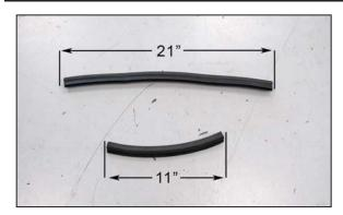
10. Cut the provided edge trim into two sections, one section will be 21" long and the shorter section will be 11" long.
