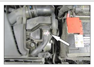
4. Cut the clamp securing the crank case vent hose to plenum and then disconnect the crank case vent hose from the plenum.
