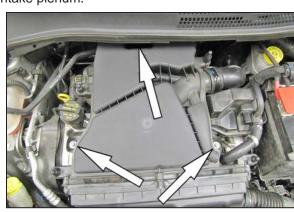
6. Loosen the three bolts securing the intake plenum to the engine.
