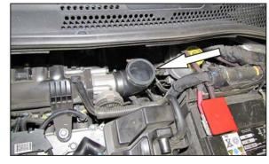
8. Install the provided elbow hose (03108) onto the throttle body as shown.
