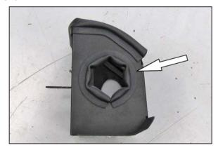
12. Install the 11" edge trim into the hole of the heat shield as shown.
