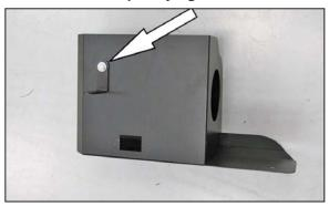
9. Install the provided "L" bracket (070662) onto the heat shield as shown.
