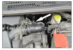
3. Loosen the hose clamp securing the intake tube to the throttle body.
