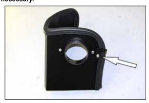
8. Install the heat shield mounting bracket (064330) onto the heat shield as shown.
