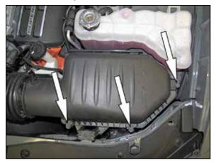
4. Loosen the three screws securing the upper air filter housing and then remove the upper air filter housing and intake tube.
