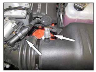
2. Disconnect the inlet air temperature sensor electrical connection and disconnect the crank case vent hose from the fitting.
