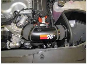
15. Install the K&N<sup>®</sup> intake tube assembly into position, Slide the coupling hoses out and onto the throttle body and filter adapter. Then adjust the tube and hoses for proper fit and secure with the provided hose clamps.
