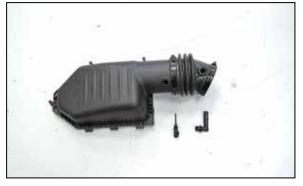
12. Remove the crank case vent and inlet air temperature sensor from the factory intake tube. **NOTE: The inlet air temperature sensor is very fragile, use car while removing the sensor.**
