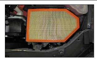
5. Remove the bolt securing the lower air filter housing to the core support and then remove the air filter housing from the vehicle.
