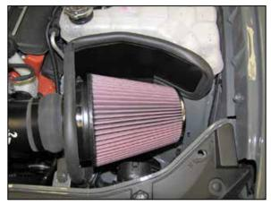
17. <u>Install the K&N air filter</u> and secure with the provided hose clamp.
