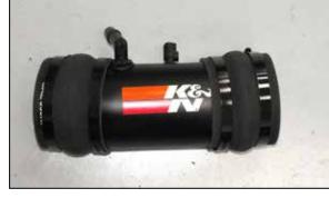
14. Install both coupling hoses (08418) onto the  $K\&N^{\otimes}$  intake tube as shown.
