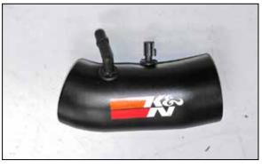
13. Install the crank case vent and inlet air temperature sensor into the K&N<sup>®</sup> intake tube. **NOTE: the inlet air temperature sensor is very fragile, use care while installing the sensor.**
