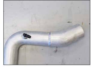
17. Install the provided 90° npt fitting into the K&N $^{\circ}$  intake tube as shown.
