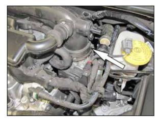
7. Loosen the hose clamp that secures the intake tube to the throttle body and then remove the intake tube from the vehicle.
