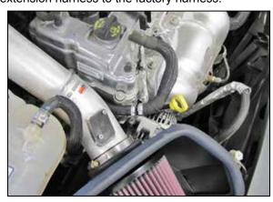
27. Connect the crank case vent hose and secure with the provided hose clamp. If the vehicle is equipped with a mass air sensor connect the electrical connection.
