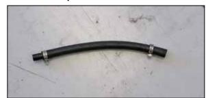
18. Install the provided hose mender into the provided crank case vent hose and secure with the provided clamp.
