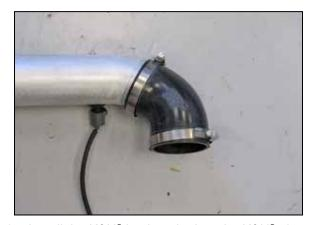
25. Install the K&N® intake tube into the K&N® air filter and then connect the coupling hose to the throttle body. Adjust the tube and hose for best fit and then secure with the provided hose clamps.
