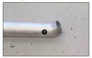
20. Install the provided grommet into the K&N® intake tube as shown.
