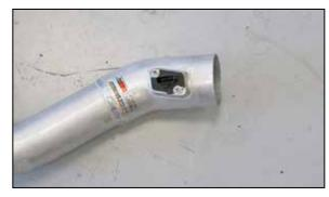
16. If the vehicle is equipped with a mass air sensor, remove the sensor from the factory housing and install it into the K&N® intake tube using the provided hardware.
