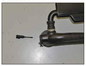
21. Remove the inlet air temperature sensor from the factory intake tube.
