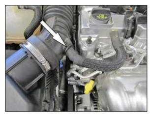
5. Disconnect the crank case vent hose from the factory intake tube.
