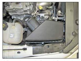
8. Lift up and remove the factory air filter housing from the vehicle.
