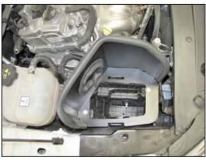
13. Install the heat shield assembly onto the lower air filter housing mount so that the mounting studs insert into the factory grommets.
