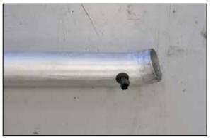
22. Remove the O-Ring from the sensor and then install the sensor into the grommet installed into the K&N intake tube.
