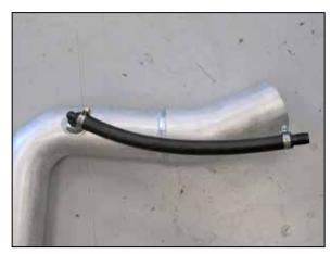
19. Install the crank case vent hose assembly onto the 90\* fitting installed into the K&N® intake tube.
