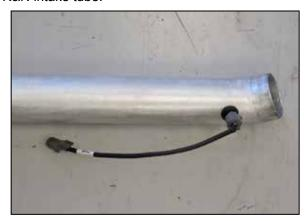
23. Install the extension harness onto the inlet air temperature sensor.
