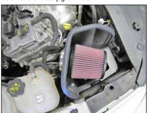
14. Install the  $K\&N^{\otimes}$  air filter through the heat shield as shown.
