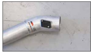
15. On vehicles that are not equipped with a mass air sensor, install the provided gasket onto the mass air sensor mount block off as shown and then install the block off onto the K&N® intake tube.
