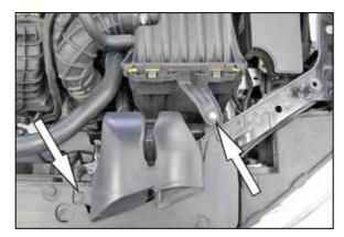
7. Loosen and remove the bolt which secures the factory air box to the core support and then remove the retaining pin securing the fresh air intake to the core support.
