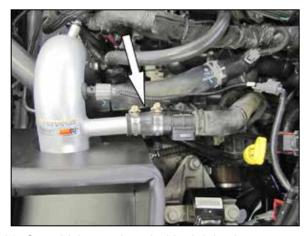
23. On vehicles equipped with air injection, connect the air injection hose to the K&N® intake tube using the provided coupling hose and clamps. On vehicles that are not equipped with air injection, install the provided cap and secure with the provided hose clamp.
