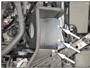
16. Install the heat shield onto the inner fender and secure with the provided hardware.
