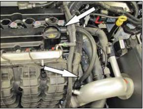
22. Install the provided crank case vent hose to the valve cover port and then connect the open end to the fitting installed into the K&N® intake tube as shown.
