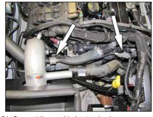
21. Connect the provided extension harness into the factory inlet air temp connector and then connect the open end to the inlet air temperature sensor. Secure the harness with the provided wire tie.
