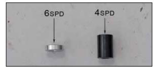
12. Choose the correct spacer to be used for the tube mounting bracket per transmission application. 4spd transmission will use the longer spacer and 6spd transmission will use the shorter spacer.
