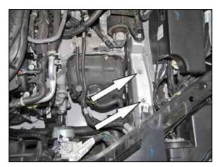
7. Remove the two air box mounting studs shown
