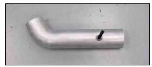
14. Install the 90° vent fitting into the intake tube
