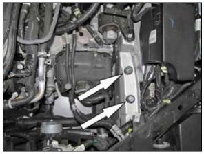
8. Install the two provided rubber mounted studs into the air box mounting stud locations.
