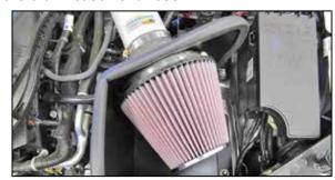
17. Install the K&N® air filter onto the filter adapter and secure with the provided hose clamp.
