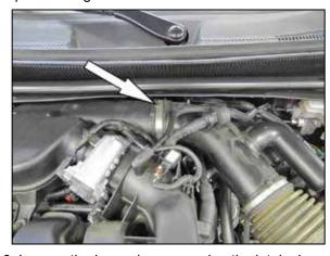
3. Loosen the hose clamp securing the intake hose to the intake plenum.
