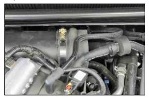
12. Install the provided silicone hose (08699) onto the intake plenum and secure with the provided hose clamp.
