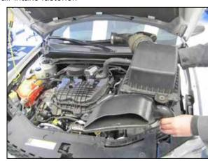
6. Lift up the complete stock intake system and remove it from the engine compartment.
