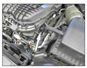
4. Disconnect the crank vent hose from the valve cover.
