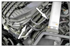
16. Install the provided crank case vent hose onto the fitting installed into the K&N® intake tube and then onto the factory fitting on the valve cover. NOTE: It may be necessary to rotate the heater hose spring clamp so that it does not contact the crank case vent hose.
