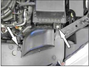
5. Remove the air box retaining bolt and the fresh air intake fastener.
