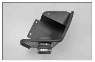
11. Install the provided silicone hose (08699) onto the filter adapter and secure with the provided hose clamp.
