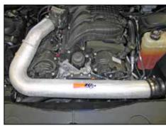
19. Install the K&N® intake tube into the silicone hump hose and then into the silicone hose on the throttle body.
