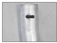
18. Install the 90° NPT fitting into the K&N<sup>®</sup> intake tube as shown.
