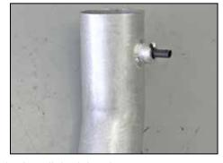
17. Install the inlet air temperature sensor into the  $K\&N^{\tiny \circledcirc}$  intake tube as shown, turning the sensor clockwise to lock.
