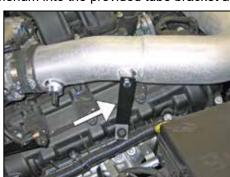
22. Install the tube bracket onto the mounting stud and then secure to the K&N<sup>®</sup> intake tube with the provided hardware. Tighten the hose clamps at this time
