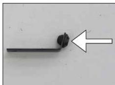
21. Install the mounting grommet from the intake plenum into the provided tube bracket as shown.
