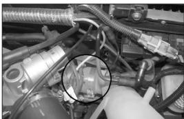
10. Tighten the hose clamp on the intake tube as shown.
