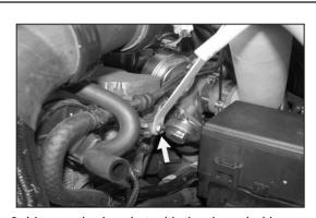
9. Line up the bracket with the threaded boss on the cylinder head and secure with the provided hex bolt.
