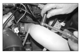
12. Slide the 2" silicone hose and hose clamp onto the vent on the intake tube and tighten as shown.
