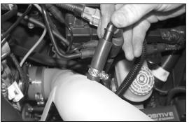
13. Reconnect the stock vent hose to the intake tube as shown.
