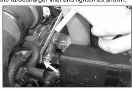
8. Slide the K&N<sup>®</sup> intake tube into the silicone hose as shown.
