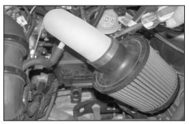
14. Install the K&N® air filter onto the intake tube and secure with the provided hose clamp as shown.
