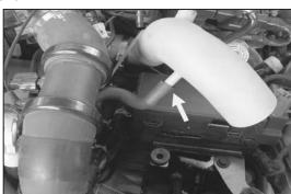
11. Remove the stock crankcase vent hose and using the supplied 10-1/2" silicone hose, measure and cut 2" off of one end of the hose and set it aside. Connect the 8-1/2" hose to the crankcase vent tube and the other end to the vent on the intake tube as shown.
