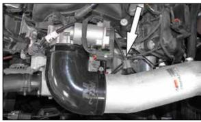
21. Connect the provided inlet air temperature sensor harness extension into the factory harness, run it under the throttle body and then connect to the inlet air temperature sensor as shown. Using the provided cable tie, secure the harness extension tube mounting bracket.
