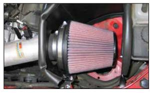
24. Install the filter assembly onto the K&N® intake tube and secure with the provided hose clamp.
