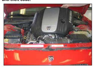
2. Lift up the engine cover to loosen it from the mounts, and then remove the cover from the vehicle.
