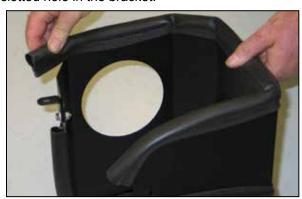
11. Install the two pieces of edge trim onto the heat shield as shown; be sure to leave a gap at the bracket mounting locations.
