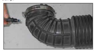
15. Remove the inlet air temperature sensor from the stock intake hose as shown.
