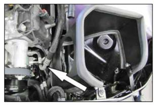
12a. Due to vehicle manufacturing tolerances, the A/C lines on some vehicles may need to repositioned slightly so that they do not contact the heat shield. To adjust, grab the A/C line on the aluminum section and carefully apply pressure in the desired direction until clearance is obtained.
