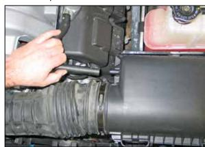
6. On SRT-8; 6.1L vehicles, disconnect the crankcase vent hose from the airbox as shown.
