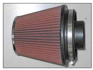
22. <u>Install the provided air filter adapter</u> into the K&N® air filter and secure with the provided hose clamp.
