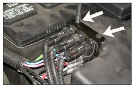
3. Loosen the two bolts that secure the solenoid bracket to the air cleaner assembly as shown.
