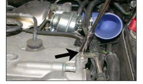
15. Remove the nut that secures the hard line to the cam cover as shown.
