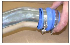
23. Slide the silicone hose and hose clamps onto the K&N $^{\odot}$  cold air tube as shown but do not tighten at this time.
