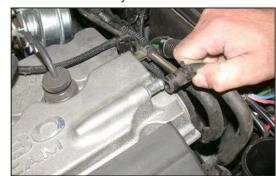
2. Loosen the hose clamp at the turbocharger inlet and at the air cleaner, then, remove the stock intake tube as shown.
