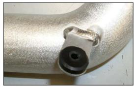
24. Insert the provided rubber grommet into the  $K\&N^{\otimes}$  cold air tube bracket as shown.
