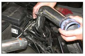
25. Slide the cold air tube into the hole in the inner fender as shown.
