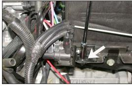
13. Mount the "L" bracket to the battery tray using the bolt removed in step 11.
