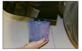
32. From underneath the vehicle install the K&N $^{\mbox{\tiny \$}}$  air filter and secure with the provided hose clamp.
