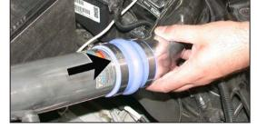
26. Line up the tube bracket with the original air cleaner mounting stud, then, slide the silicone hose onto the short ram tube as shown.
