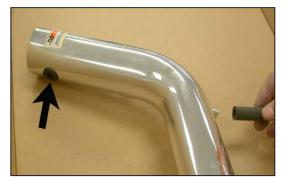
16. Install the provided grommet into the hole on the K&N $^{\circ}$  short ram tube.
