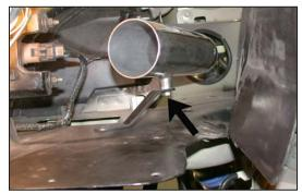
29. From underneath the vehicle install the "Z" bracket onto the threaded boss on the intake tube as shown but do not tighten at this time.
