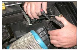
6. Remove the air temperature sensor from the air inlet duct as shown.
