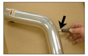
17. Cut a 2" length and a 4-1/2" length of silicone hose from the provided 10" length of silicone hose and install the 2" length hose onto the K&N<sup>®</sup> intake tube as shown.
