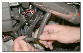
22. Slide the silicone hose onto the vent on the  $K\&N^{\otimes}$  short ram tube, then connect the 90 degree vent to the stock vent as shown.
