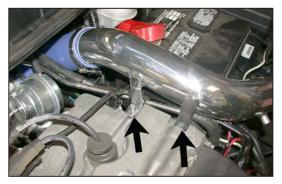
18. Slide the K&N<sup>®</sup> short ram tube into the silicone hose, then line up the tube bracket with the stud on the cam cover while sliding the silicone hose onto the vent on the cam cover as shown.
