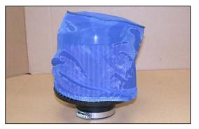
31. Slide the K&N $^{\circ}$  Drycharger $^{\circ}$  onto the K&N $^{\circ}$  air filter as shown.
