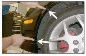
28. Remove the two screws that secure the inner wheel valance using a torx, size T25 as shown.
