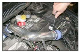
35. Adjust everything for best fit and clearance, then, tighten all hardware and hose clamps as shown.
