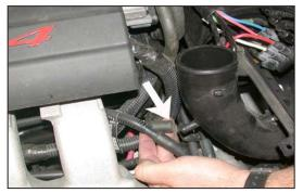
9. Disconnect the vent on the air cleaner tube as shown.
