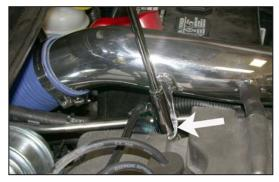
19. Secure the tube bracket to the cam cover stud using the nut removed in step 15 but do not tighten at this time.
