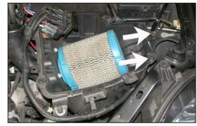
7. Remove the bolt and nut that secure the lower air cleaner assembly to the inner fender as shown.
