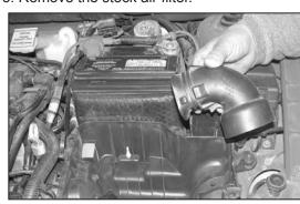
6. Pull up and remove the fresh air intake from fender well.
