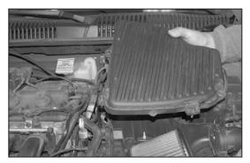
4. Loosen and remove the five air box retaining bolts then remove air box lid as shown.
