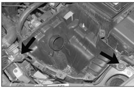
9. Remove the bolt and nut that secure the the air box to the vehicle. Bolt will be re-used.
