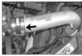
23. Slide the intake tube down the resonator hole then insert the other end into the throttle body silicone hose.
