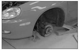
11. Jack the driver's side of the vehicle up and support with jack stands then remove the tire.
