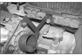
17. Using the battery tray mounting bolt that was removed in step 15, mount the throttle body bracket to the battery tray as shown.
