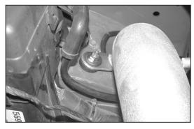
25. Using the supplied nut, tighten the intake tube bracket to the stock stud.
