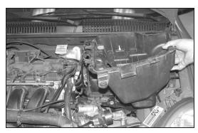
10. Remove the air box from the vehicle.
