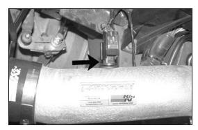
27. Install the air temp. sensor into the rubber grommet on the K&N<sup>®</sup> intake tube.
