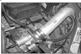
28. Using the supplied silicone hose, attach one end to the K&N<sup>®</sup> intake tube and the other end to the crank case vent tube.
