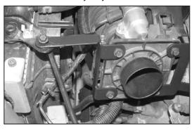
18. Using the stock bolt removed in step 9, secure the throttle body bracket to the stock air box mount.
