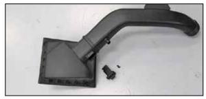
14. Remove the two screws securing the mass air sensor into the factory intake tube and then remove the mass air sensor from the housing.
