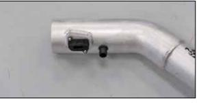
15. Install the mass air sensor into the K&N $^{\odot}$  intake tube and secure with the provided hardware.
