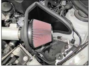
18. Install the K&N<sup>®</sup> air filter and secure with the provided hose clamp.
