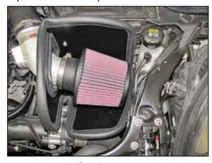
16. Install the K&N® air filter onto the intake tube and secure with the provided hose clamp. Adjust the tube and filter position for best fit.
