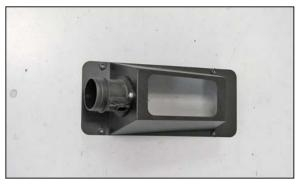
8. Remove the O-ring from the mass air sensor and then install the mass air sensor to the K&N® heat shield and secure with the provided hardware.
