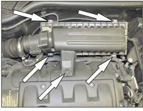
5. Loosen the one bolt and four screws that secure the upper air filter housing.
