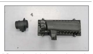
7. Remove the two bolts that secure the mass air sensor to the upper housing and then remove the mass air sensor.
