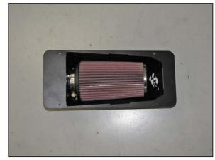
9. Install the K&N<sup>®</sup> air filter onto the mass air sensor and secure with the provided hose clamp.
