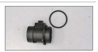
7. Remove the factory O ring from the mass air sensor.
