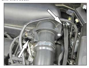
2. Disconnect the mass air sensor electrical connection and unhook the vent line from the air box.
