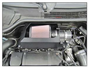
12. Install the K&N® heat shield assembly onto the factory lower air box and secure with the factory bolts from step #12.
