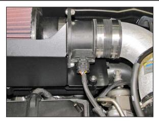
14. Reconnect the mass air sensor electrical connection.
