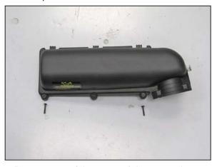
11. Remove two of the upper air box mounting bolts as shown.
