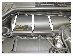
4. Loosen the three screws securing the upper air box housing to the lower housing
