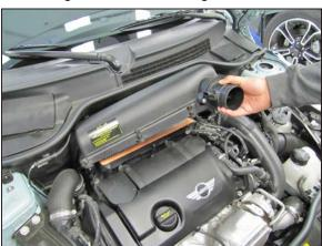
5. Remove the upper air box housing and air filter from the vehicle.
