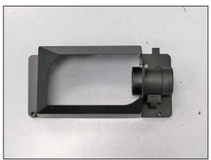
8. Install the mass air sensor into the K&N® heat shield using the provided hardware.
