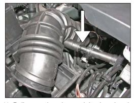
11. Pull upward on the stock intake tube, then, using a pair of pliers disconnect the stock crank case vent hose from the stock intake tube as shown.
