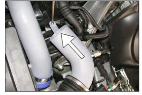
28. <u>Install the new air inlet tube</u> into the stock air inlet duct, then, line up the bracket with the hole on the lower air cleaner assembly and secure with the provided screw as shown.
