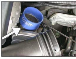
19. Install the silicone hose and the provided hose clamp onto the throttle body and tighten as shown.
