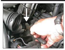
10. Using a pair of dikes or pliers, unclip the stock hose clamp on the stock intake tube at the throttle body as shown.
