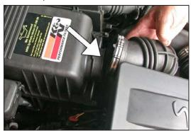
3. Pull the stock intake tube off the air cleaner as shown.
