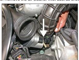
9. Remove the throttle body electrical connection as shown.
