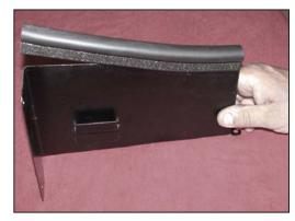
15. Install the provided edge trim onto the K&N<sup>®</sup> heat shield as shown.
