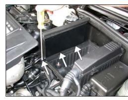
16. Install the heat shield onto the top edge of the lower air cleaner assembly, then, secure the front tab of the heat shield to the lower air cleaner assembly using the provided screw as shown.
