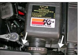
5. Loosen the two bolts on the front of the air cleaner assembly as shown.
