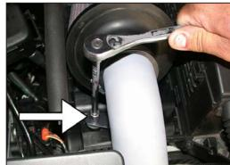
24. Using the provided hardware secure the "Z" bracket to the rubber mounted stud as shown.
