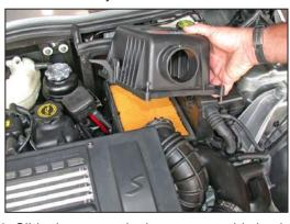
6. Slide the upper air cleaner assembly backwards, then, pull upward to remove the upper air cleaner assembly as shown.
