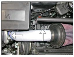
23. Install the intake tube assembly into the silicone hose at the throttle body, then, line up the bracket with the rubber mounted stud as shown.
