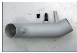
19a. On vehicles that come equipped with the additional vent line, install the provided vent fitting into the intake tube as shown. On all others install the provided plug.
