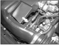
3. Using a pair of side cutters cut the factory hose clamps on the stock intake tube at the throttle body and at the air cleaner assembly as shown.
