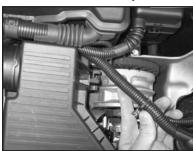
6. Using a pair of needle nose pliers unclip the electrical harness from the side of the airbox assembly as shown.
