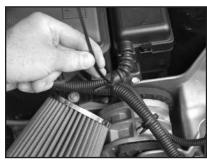
18. Secure the harness away from the air filter using a provided plastic tie as shown.
