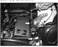
7. Models between April 2001-2004: Remove the two bolts that secure the air cleaner assembly as shown.
