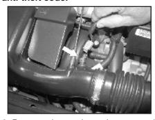
2. Remove the stock crankcase vent hose from the cam cover as shown.
