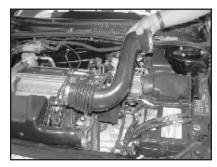
5. Remove the harness multi plug from the side of the air cleaner assembly.
