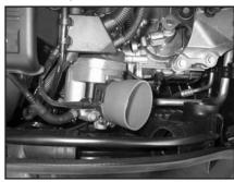
11. Secure the silicone stepped hose and hose clamps onto the throttle body as shown.
