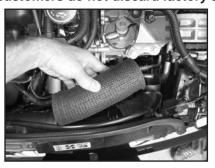
10. Remove the foam feed pipe from between the intake scoop & resonator box as shown.
