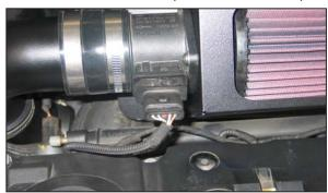
17. Reconnect the mass air sensor electrical connection.
