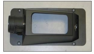
11. Using the provided hardware, secure the factory mass air sensor to the K&N® heat shield as shown.
