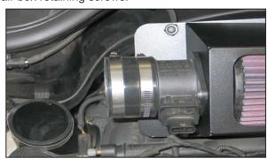
15. Install the provided silicone hose (08756) onto the mass air sensor and secure with the provided hose clamp.
