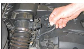
2. Release the locking tab and then disconnect the mass air sensor electrical connection.
