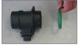
9. Remove the "O" ring from the mass air sensor as shown.
