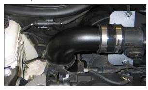
16. Install the K&N® intake tube into the silicone hoses and secure with the provided hose clamps.
