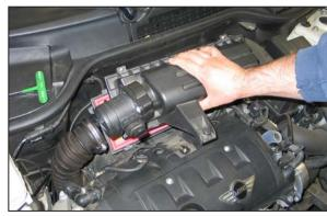
6. Remove the upper air box from the vehicle as shown and then remove the stock air filter.
