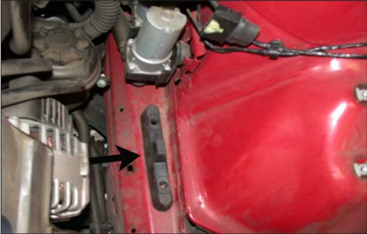
11. Remove the rubber air cleaner grommet by pulling firmly upwards.
