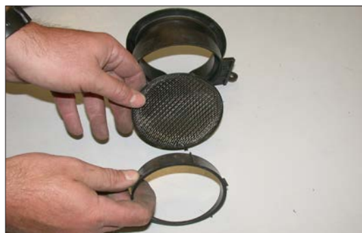
19. Disassemble the velocity stack as shown.
