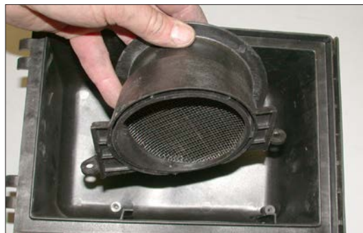
18. Remove the velocity stack from the inside of the air cleaner cover, which is secured by two screws.
