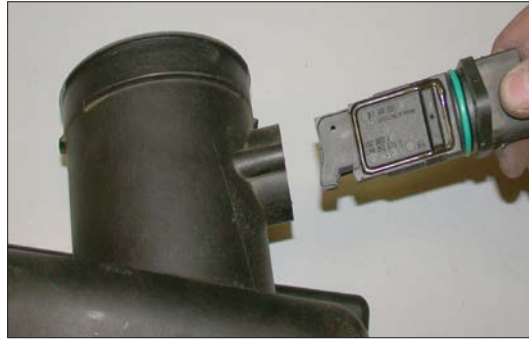
17. Using the supplied T-20 torx wrench, remove the mass air sensor from the air cleaner cover as shown.
