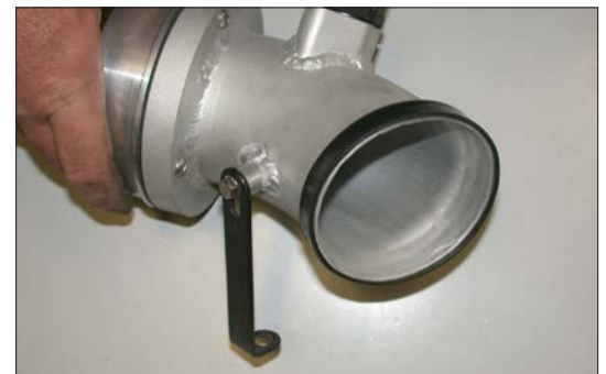
25. Install the provided bracket onto the intake tube assembly using the provided hardware as shown.
