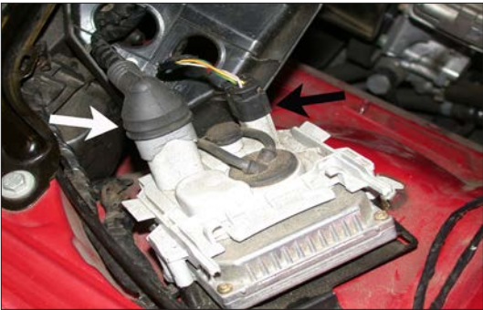
12. Reconnect the electrical connections to the high intensity discharge unit as shown.
