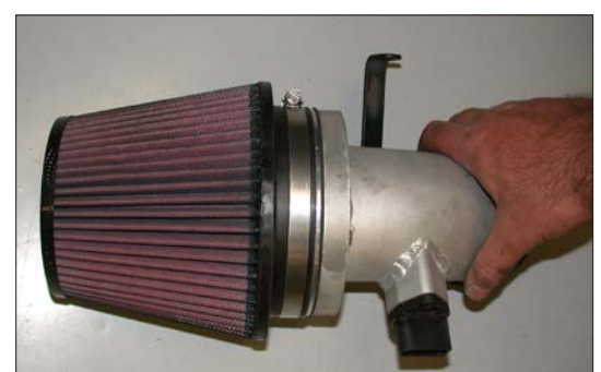
26. Install the air filter onto the intake tube assembly and secure with the provided hose clamp as shown.
