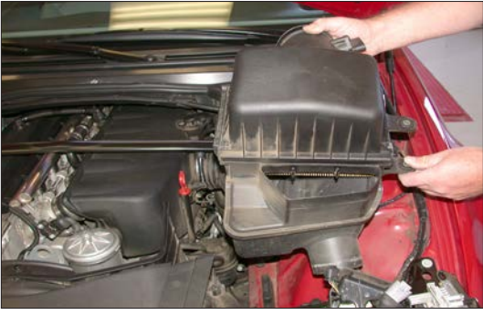
10. Pull firmly upwards to remove the air cleaner as shown.
