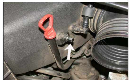
27. Remove the cap nut from the dipstick tube as shown.
