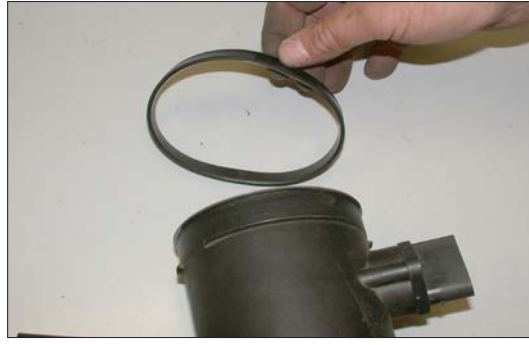
16. Remove the rubber seal from the air cleaner flange as shown.
