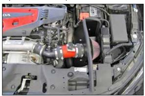
14. Install the intake tube assembly onto the turbo inlet and filter adapter, adjust the tube for best fit and secure with the provided hose clamp.
