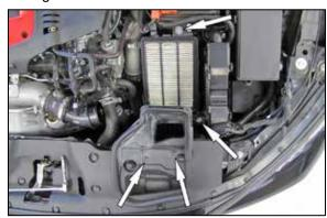
4. Remove the four bolts that secure the lower air filter housing and fresh air scoop and then remove the complete assembly from the vehicle.
