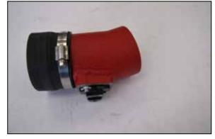
12. Install the provided coupler (084091) onto the inlet side of the K&N® intake tube and secure with the provided hose clamp.
