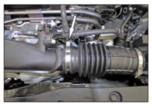
3. Loosen the hose clamp that secures the intake hose to the turbo inlet.
