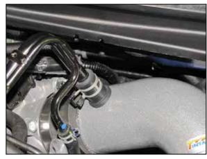
21. Insert the crankcase vent tube into the grommet installed into the K&N<sup>®</sup> intake tube and use the factory spring clamp to secure.
