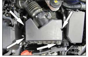
4. Loosen the four screws securing the upper air filter housing and disconnect the wiring harness from the housing.
