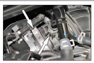
3. Release the spring clamp securing the crank case breather tube and then loosen the hose clamp that secures the intake tube to the throttle body.
