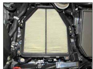
6. Remove the factory air filter.
