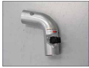
18. Remove the mass air sensor from the factory air filter housing and install it into the K&N<sup>®</sup> intake tube using the provided hardware.
