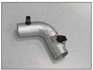
19. Install the provided grommet into the K&N<sup>®</sup> intake tube along with the factory crank case vent spring clamp.
