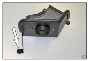
11. Remove the factory air filter housing mounting grommet from the factory air filter housing and install it into the K&N® heat shield as shown.
