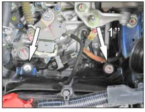
12. Install the two provided rubber mounted studs into the factory air filter housing mounting locations. NOTE: The longer 1" mounting stud is to be installed into the outer most location.
