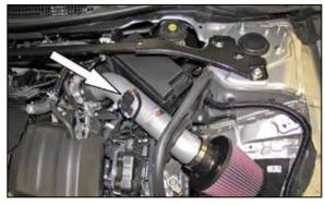
19. Reconnect the mass air sensor electrical connection.
