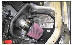
18. Install the K&N<sup>®</sup> air filter onto the K&N<sup>®</sup> intake tube and secure with the provided hose clamp
