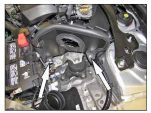
9. Install the heat shield onto the factory air box mounting locations and secure with the provided hardware.
