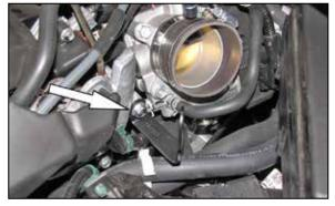
14. Install the provided tube mounting bracket (064308) onto the engine as shown using the bolt from the previous step.
