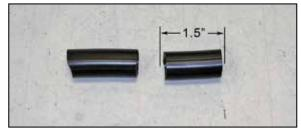
16. Cut the provided crank case vent hose to a length of 1-1/2" long as shown.
