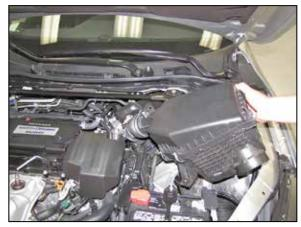
6. Remove the complete factory intake system from the vehicle.
