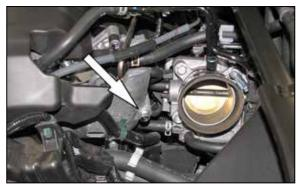
13. Remove the bolt shown from the engine; this bolt will be reused in the next step.
