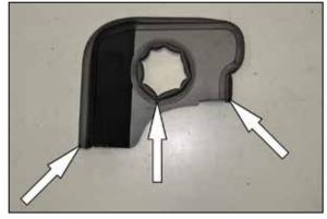
8. Install the edge trim into the hole and around the outside of the heat shield as shown.
