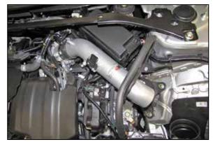
15. Install the K&N<sup>®</sup> intake tube through the heat shield, into the silicone hose at the throttle body and align with the mounting bracket. Secure the tube with the provided hardware and hose clamp.
