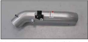
12. Install mass air sensor into the K&N<sup>®</sup> intake tube and secure with the provided hardware.
