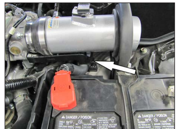
21. Using the provided tie wrap, Secure the wiring harness to the tube mounting bracket.
