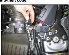
2. Disconnect the mass air sensor electrical connection and then unhook the wiring harness from air box.
