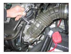
3. Release the spring clamp and then disconnect the crank case vent hose from the intake tube.
