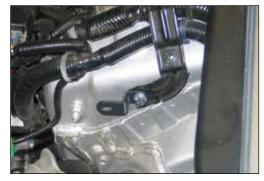
15. Install the heat shield mounting bracket (070061) onto the air box mounting bracket and secure with the provided hardware.
