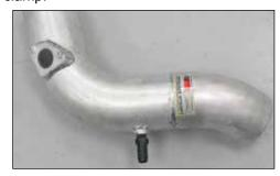
20. Install the provided vent fitting into the K&N® intake tube as shown.
