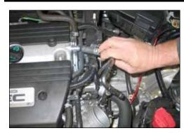
Release the spring clamp which secures the crank case vent hose to the valve cover and then unhook crank case vent hose from the valve cover as shown.
