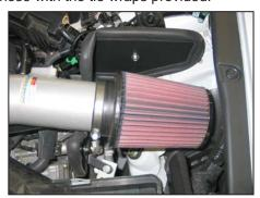
21. Install the K&N® air filter onto the intake tube and secure with the provided hose clamp.
