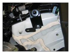
11. On Honda vehicles, install the heat shield mounting bracket (070116) onto the air box mounting bracket and secure with the provided hardware.
