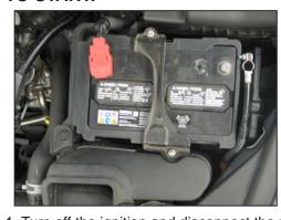
1. Turn off the ignition and disconnect the negative battery cable.
