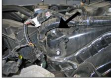
11a. On Acura vehicles Install the heat shield mounting bracket (083158) onto the strut tower and secure with the provided hardware.
