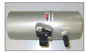
18. Install the mass air sensor into the K&N<sup>®</sup> intake tube and secure with the provided hardware.
