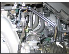
4. Disconnect the crankcase vent tube from the intake tube and valve cover port as shown. The spring clamps will not be reused.
