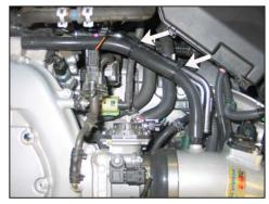
20. Install the provided crankcase vent hose onto the NPT fitting and then onto the valve cover port. Secure the crankcase hard line to the provided hose with the tie wraps provided.
