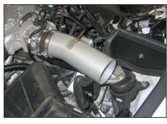
19. Install the K&N® intake tube into the silicone hose at the throttle body and align with the mounting bracket. Secure with the hose clamp and provided hardware.
