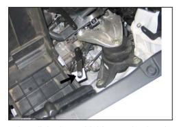
12. Install the heat shield mounting bracket (070115) onto the airbox mounting location on the battery tray using the provided hardware.
