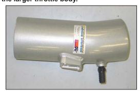
16. Install the  $1\!\!/\!_4$  NPT fitting into the K&N® intake tube as shown.
