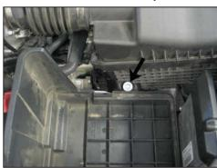
6. Loosen the bolt which secures the lower airbox to the battery tray.
