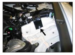
10. On Honda vehicles, remove the airbox mounting bracket bolt shown.
