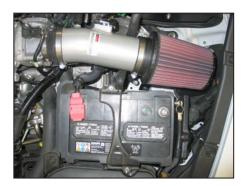
22. Reinstall the battery and secure with the hold down bracket. Reconnect the positive battery cable.
