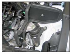
14. Install the heat shield assembly into the vehicle and secure to the mounting brackets with the hardware provided.
