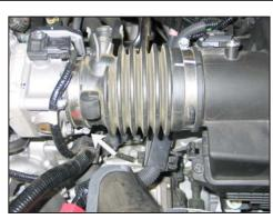
5. Loosen the hose clamp which secures the stock intake tube to the throttle body.
