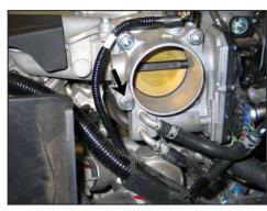
8. Remove the front lower throttle body bolt shown. **NOTE: This bolt will be reused in the next step.**
