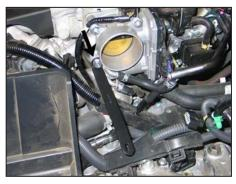
9. Install the tube mounting bracket (070114) onto the throttle body and secure with the bolt removed in the previous step.
