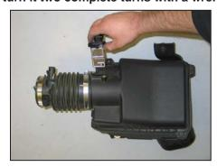
17. Remove the mass air sensor from the stock airbox.
