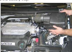
7. Remove the airbox assembly from the vehicle; be sure to unhook the wiring harness from the airbox as it is removed.
