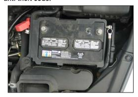
2. Disconnect the positive battery cable, remove the battery hold down and then remove the battery.
