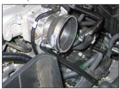
15. Install the silicone hose (084093) onto the throttle body and secure with the provided hose clamp
