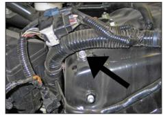
10a. On Acura vehicles, remove the bolt shown that secures the wiring harness mounting bracket to the strut tower.
